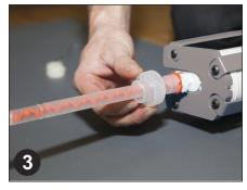
Install the mixing nozzle and secure with the previously removed cap.
