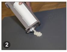
Using a piece of cardboard or scrap Protect-All, dispense the Protect-All Rapid Weld until Part A (white) and Part B (color) flow from the end.
