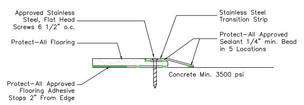
Note 1: Flooring must be routered prior to installation for smooth, flat transition
