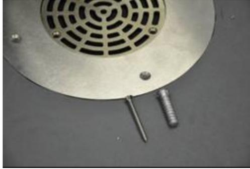
**Image 28:** Secure drain ring or transition strip to substrate. Only use #10 2-½” or #12 1-¼” stainless steel screws (tapered head) with lead anchors
